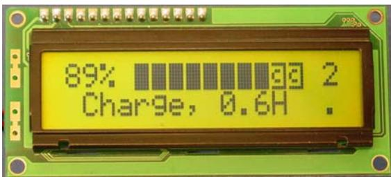
**Figure 24: Time to fully charged complete display
