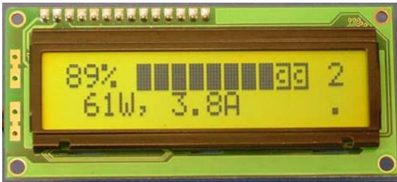
**Figure 22: Power and Current entering batteries display
