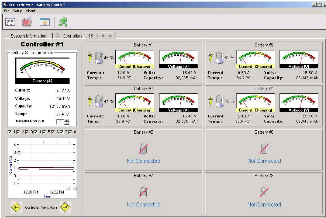
Figure 6: This screen capture shows the same four batteries and the state of charge after 70 minutes.
